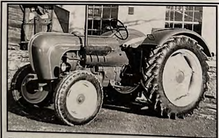
The 40s and 50s saw an ingenious proliferation of Porsche vehicles. A tractor with a two-, three- or four-cylinder aluminum engine was a short-lived but popular project. Other vehicles included an all-wheel drive light off-roader, a hunting vehicle as well as a curiously amphibious vehicle complete with rear screw for nautical mobility.
